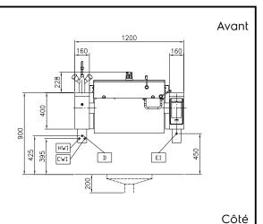
CWII Raccordement eau froide HWI = Raccordement eau chaude D
